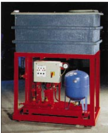
A typical fire hose reel booster system, with overhead suction tank in compliance with British Standard code of practice BS 5306 Pt. 1.
